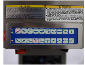
Back lit back-up controls for emergency situations
