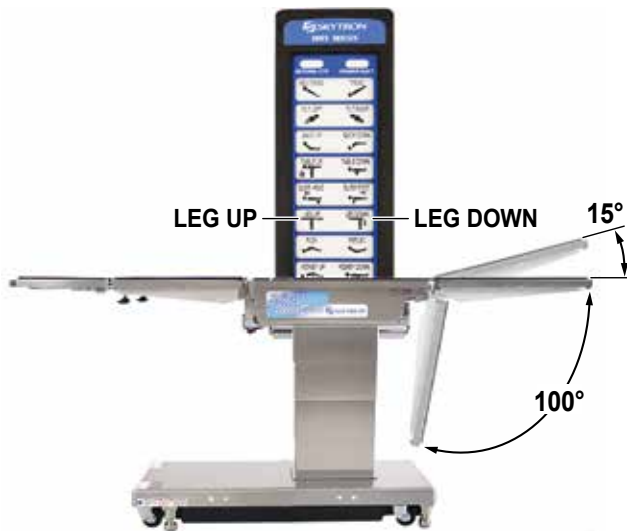
Figure 18. Leg Section Positioning
