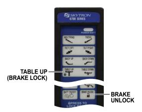
Figure 3-10. Brake System Activation
