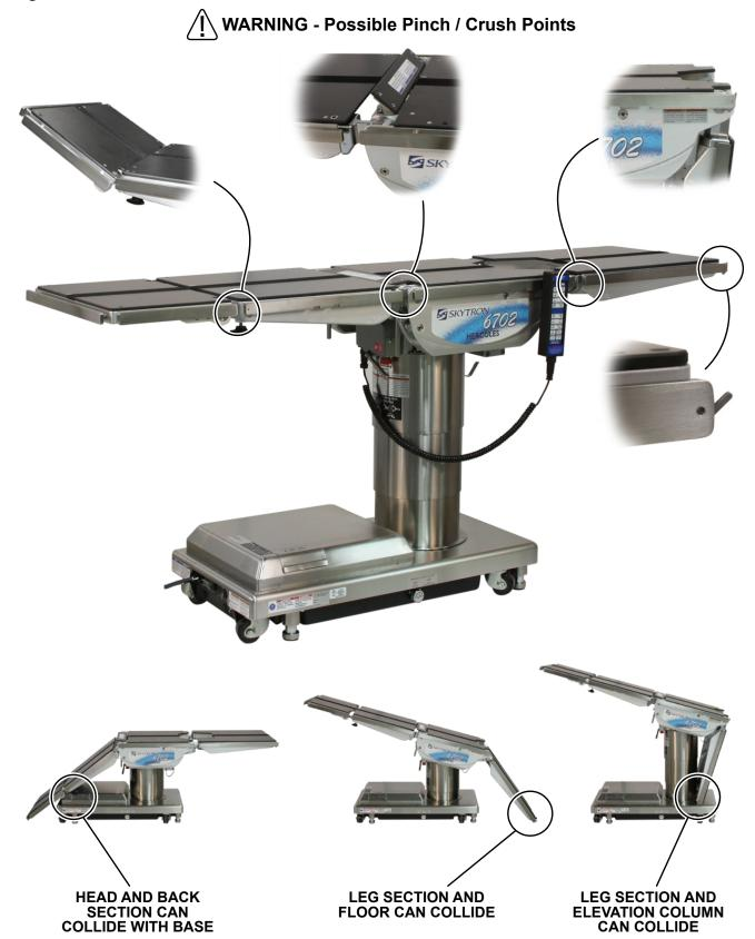
Figure 1-1. Possible Pinch or Crush Points
