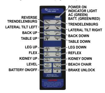
Figure 3-8. Pendant Control Function Buttons
