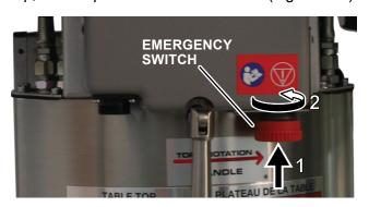
Figure 3-20. Emergency Stop Switch
