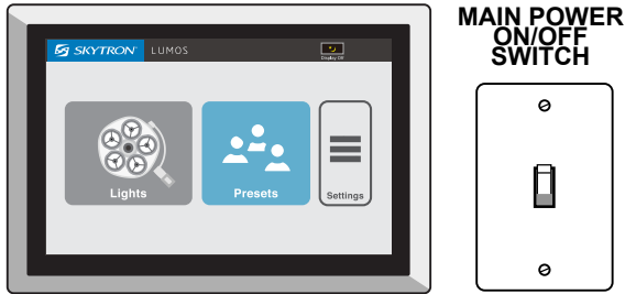
Figure 11. Control panel & main power switch
