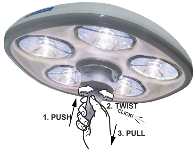
Figure 9. Sterilizable handle installation
