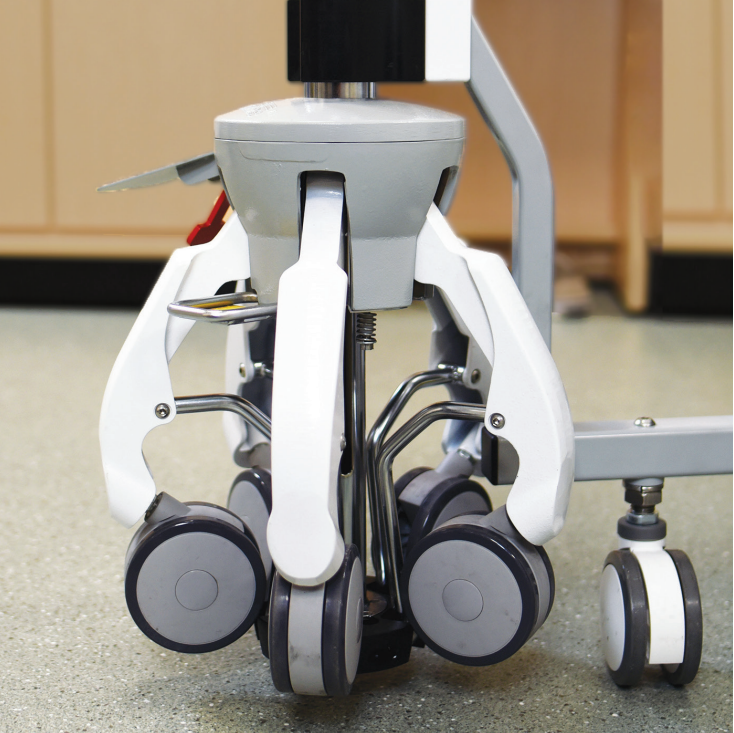
The Suspension Stand is now securely locked and off the ground.
